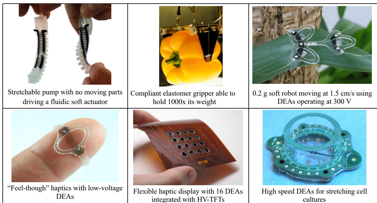
Fig. 1. Examples of high-performance elastomer-based actuators.
